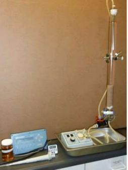
Figure 5: Ion Exchange Resin Test Apparatus
