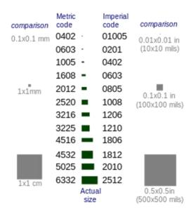
Figure 1: Passive Component Miniaturization
