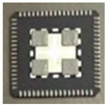
Figure 8: Preforms at the Corners of the Ground Pad
