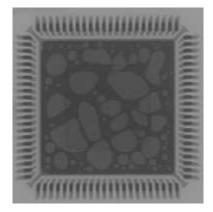
Figure 4: Large Voids due to Restricted Channels for Flux Volatiles to Outgas
