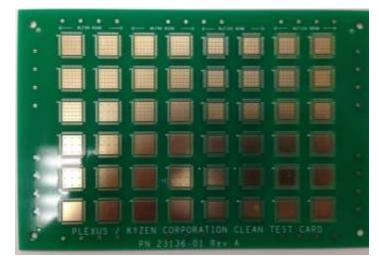
Figure 11: Test Vehicle used for this Research Study
