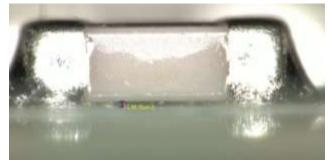
Figure 2: Passive Component Standoff Gap Example
