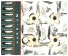
Figure 9: Plated Via Holes in Ground Pad
