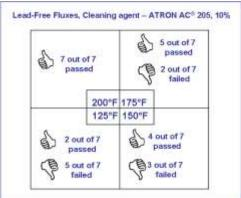
Figure 7: Cleaning results at various operating temperatures
