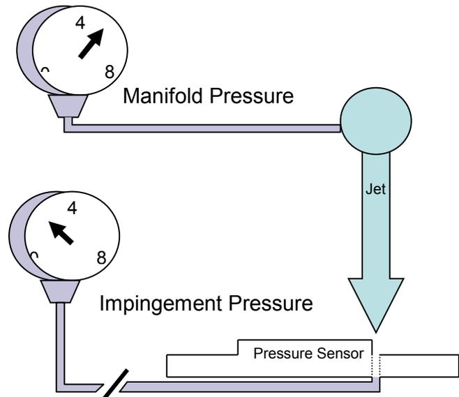
The manifold pressure sensor will be setup to differentiate manifold pressure from impingement pressure. Note; size the opening of the pressure sensor to match as closely as possible the true gap dimensions of the component.
