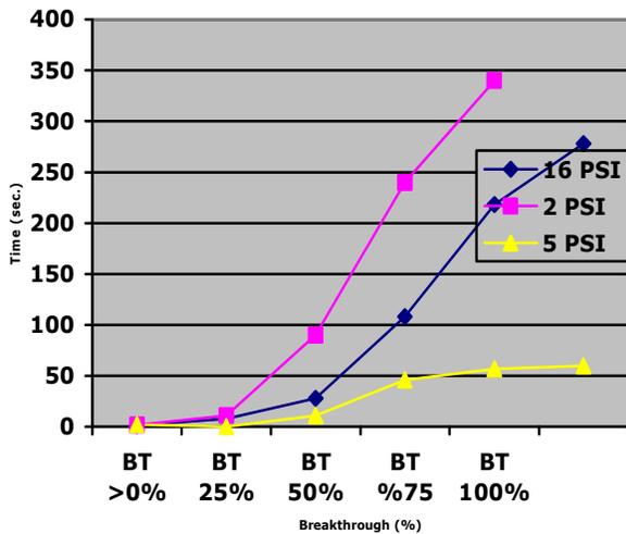
**Figure 7:** Observed effect of to high pressure jet spreading in 3-D pattern versus 2-D surface spread on lower pressure jet
