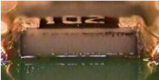
Drivers for removing all flux residues under component include time in the wash section, nozzle type, pressure, cleaning fluid, and temperature. The limiting factor is time. Data findings from designed experiments indicate 5-15 minutes is required in the wash section to remove all flux residues under low standoff component.
