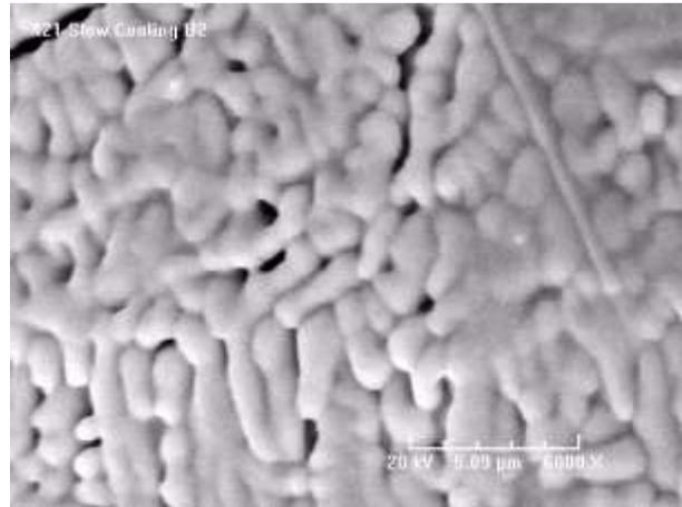
Fig. 3 Surface dendrite structure of Sn95.5Ag3.5AgCu1.0 solder joint [9].
