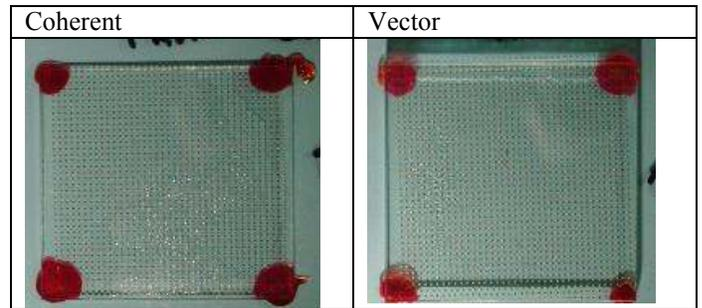
Figure 10 illustrates improved cleaning data findings of coherent versus vector jets using a longer wash time of four minutes. The following parameters were tested:
