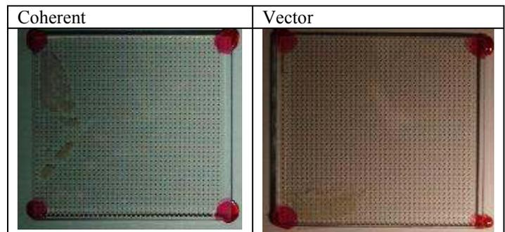
Figure 7 illustrates the data findings of coherent versus vector jets using a longer wash time of six minutes using the following process parameters:
