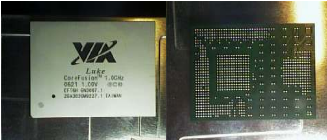
Photo 1: Overview of control test vehicle soldered w/ ws609.
