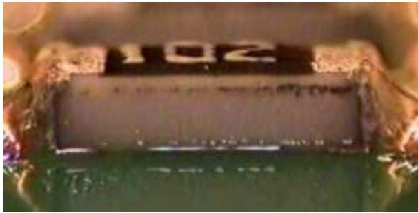
Figure 1: Flux residue trapped under component
