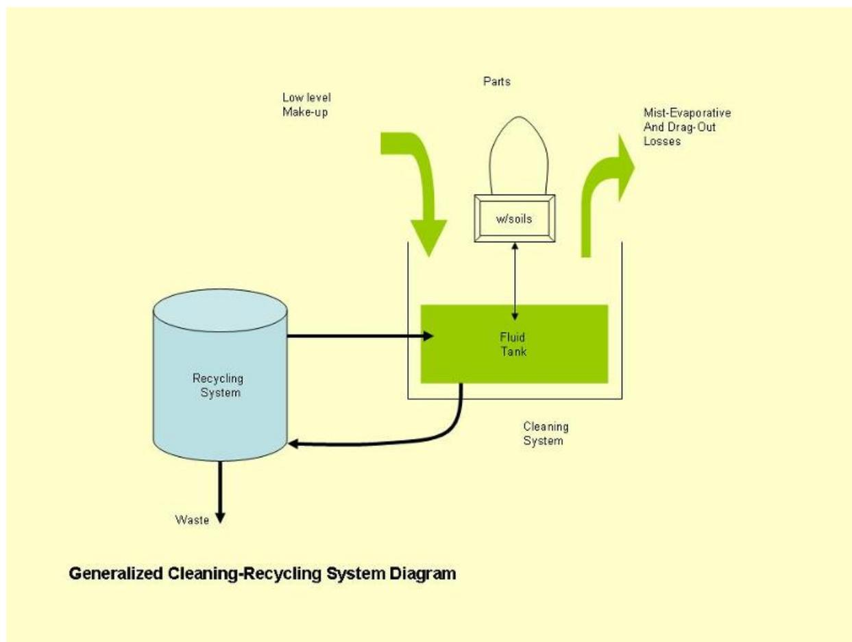
Figure 1; Mass balance diagram of a generalized cleaning process equipped with a solvent recycling system.
