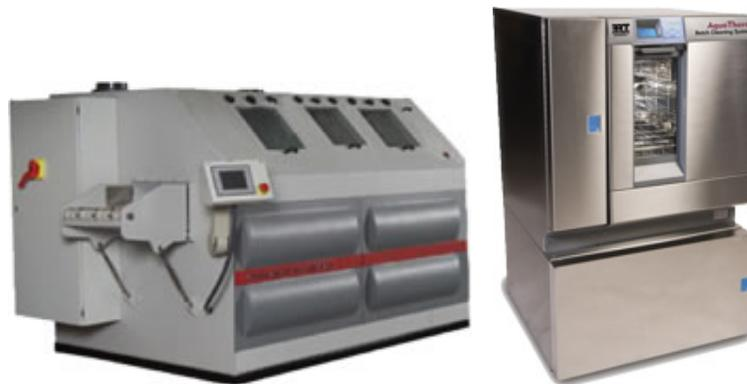
Burnet TX - Austin American Technology Corporation is offering new super compliant cleaning systems for circuit board de-fluxing. The new cleaners have been designed to be used with super compliant cleaning agents as defined by the South Coast Air Quality Management District (SCAQMD) and the anticipated new guidelines coming from the Ozone Transportation Commission (OTC) for the US East Coast.
