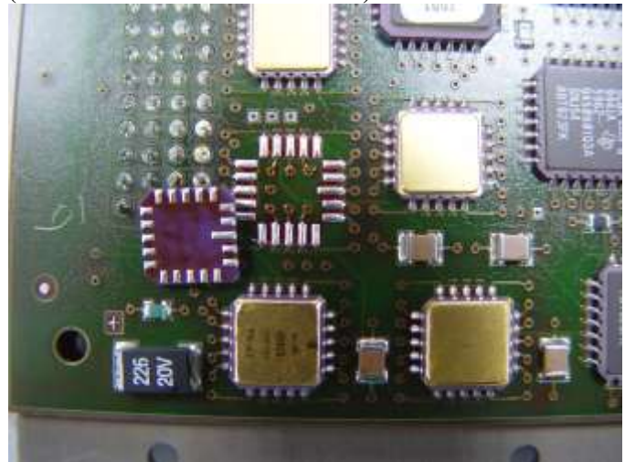
Figure 1: Heavily populated with Leadless Chip Carriers (one removed to show flux residue)
