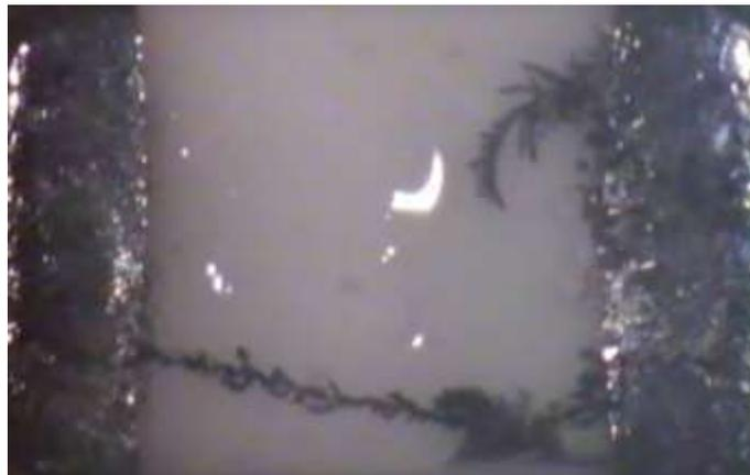
Figure 5: Flux Bridging Conductors can lead to ECM
