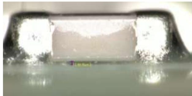
Figure 2: Passive Component Standoff Gap Example
